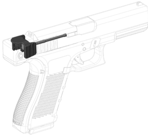
Figure 7: Location of the RCD inside the pistol slide.
