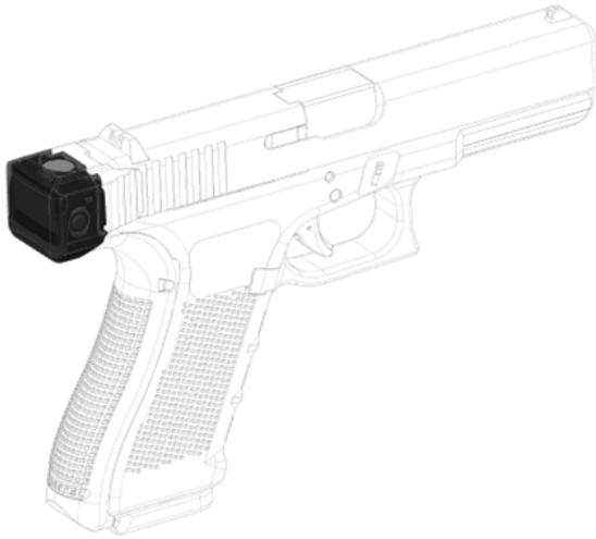
Figure 13: Location of the RISC Display in the pistol.
