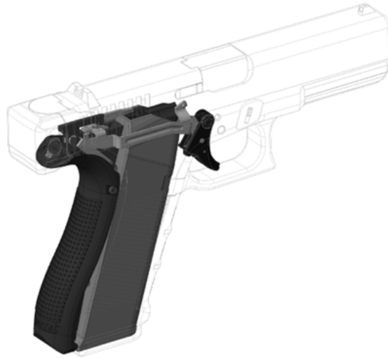
Figure 9: Location of the Smart Magazine inside the pistol frame.
