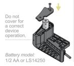
Attach DIGITAL COUNTER counter device to the lower receiver using screws and washers from the package
